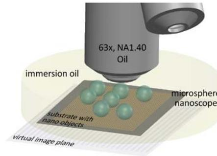
Figure 1. Schematic of the super-resolution imaging setup.
