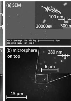
Figure 4. Measurement of gold nanorods with axial diameter of  $50\ \text{nm}$  and length of  $100\ \text{nm}$ , by both SEM and optical microscopy with a microsphere.
