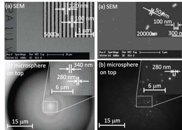
Figure 3. Measurement of nanolines with a width of  $120\ \text{nm}$  and inter-space of  $100\ \text{nm}$ , by SEM and optical microscopy with a microsphere.
