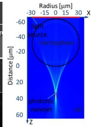
Figure 5. FEM simulation on the light propagation through a microsphere and immersion oil, showing that the light is highly focused into a photonic nanojet.
