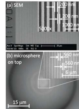
Figure 2. Measurement of nanolines with a width of  $200\ \text{nm}$  and inter-space of  $200\ \text{nm}$ , by both SEM and by optical microscopy using a microsphere in combination with an oil immersion objective.
