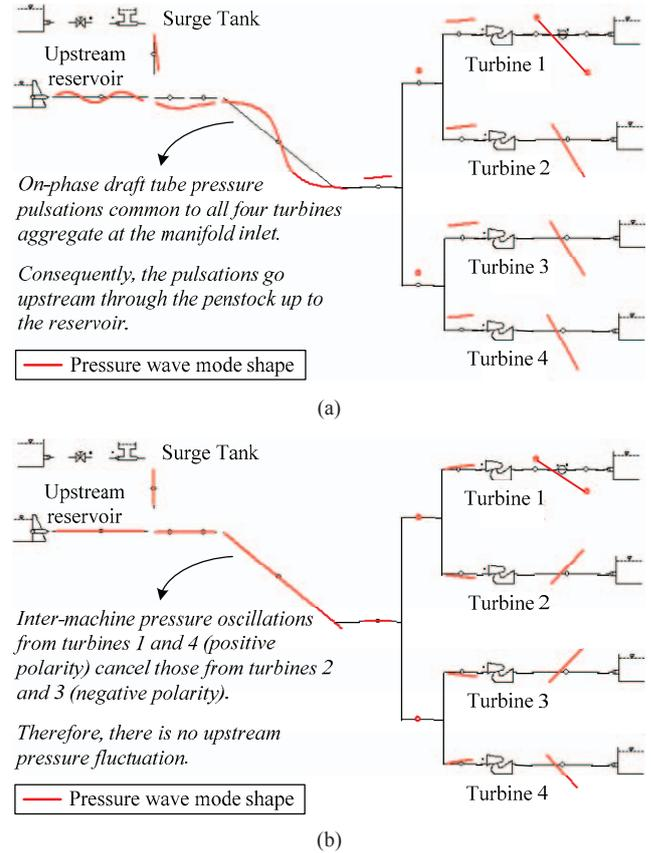
Fig. 5. Draft tube 2<sup>nd</sup> elastic common (a) and inter-machines (b) modes.
