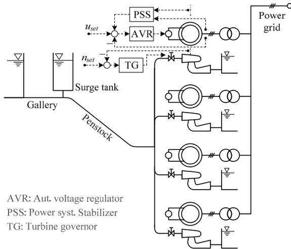
Fig. 1. Layout of the hydroelectric power plant [13].
