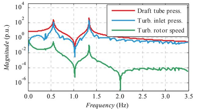
Fig. 6. Forced response of the hydraulic system.
