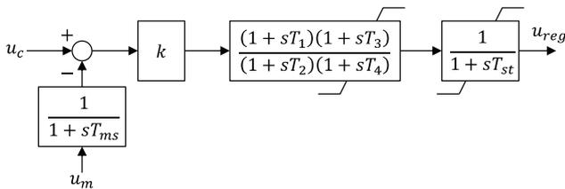
Fig. 2. Transfer function of the ABB UNITROL<sup>®</sup> voltage regulator.
