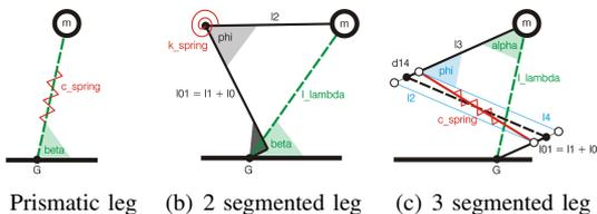
Fig. 1. Schematic presentation of compliant legs; (a) prismatic, (b) two segmented, (c) three segmented pantograph.
