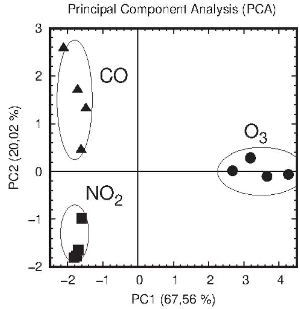
Fig. 5. PCA scores plot of the quantity  $f \cdot (S_{\delta_{\text{sensor}}}(f) - S_{Th}(f))$  for four concentrations of ozone ( $O_3$ ), nitrogen dioxide ( $NO_2$ ) and carbon monoxide (CO) detected by metal-oxide gas microsensor with tungsten trioxide ( $WO_3$ ) sensing layer.
