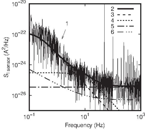
Fig. 2. Spectral decomposition of a noise response under CO (10 ppm): measurements (curve 1), total noise (curve 2), adsorption-desorption noise modeled by two Lorentzians (curve 3 and 4), white noise proportional to the resistance of the sensor (curve 5); extracted noise model of low-noise current preamplifier (curve 6).
