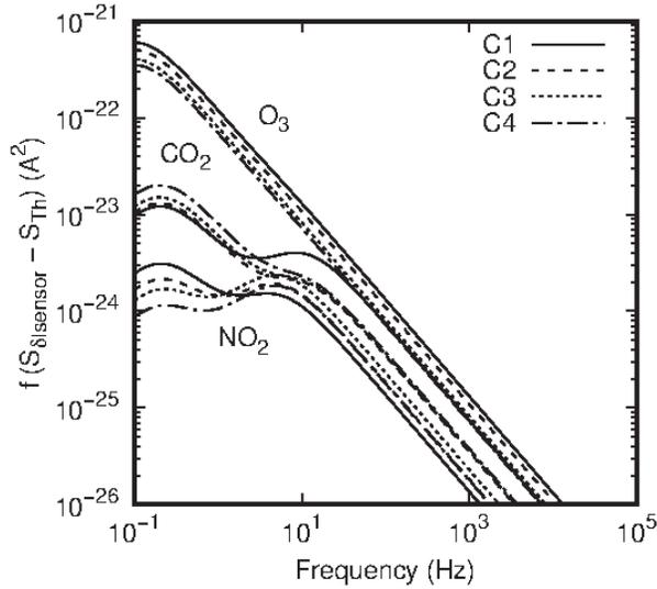
Fig. 4. Plots of the quantity  $f \cdot (S_{\delta_{\text{sensor}}}(f) - S_{Th}(f))$  for four concentrations of ozone ( $O_3$ ), nitrogen dioxide ( $NO_2$ ) and carbon monoxide (CO) detected by metal-oxide gas microsensor with tungsten trioxide ( $WO_3$ ) sensing layer.
