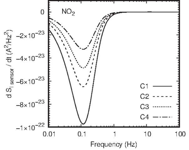
Fig. 3. Plots of the first derivative of noise current spectral density of the four concentrations of nitrogen dioxide.
