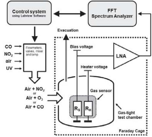
Fig. 1. General diagram of measurements setup used to characterize microsensors noise responses
