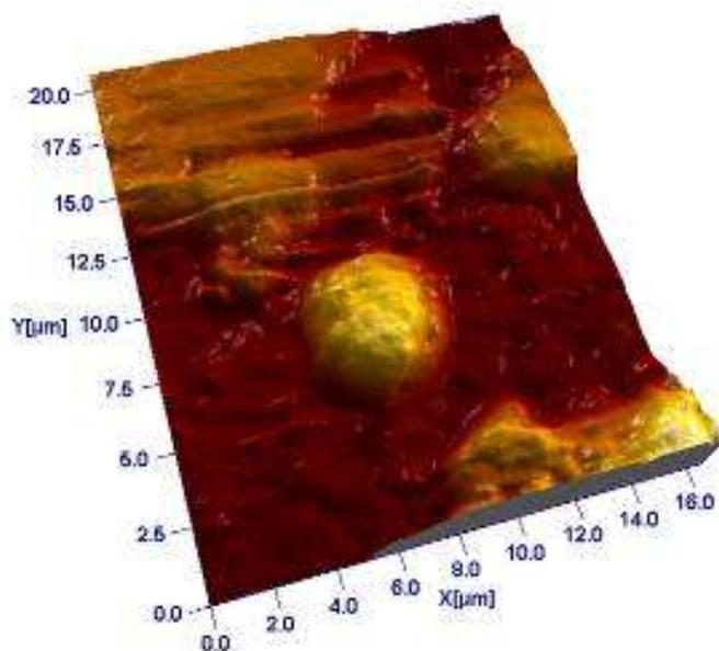
FIG. 2. AFM image taken on August 17<sup>th</sup> 2008 on sol 82 of the Phoenix mission. This dustfall sample shows a spheroidal particle (in the center) and more platy particles on the top side.
