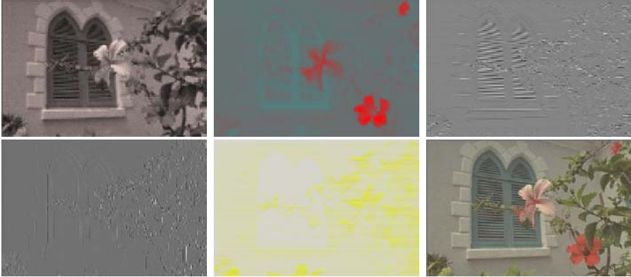
Fig. 3. Partial reconstruction of the original image (Figure 2) using only a few basis functions. (Top) Using the first, the second, and the third basis function. (Bottom) The reconstruction using the fifth, the seventh, and using first through seventh basis functions
