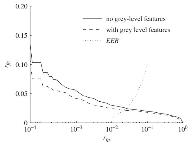
Fig. 5. Influence of grey-level features.  $\overline{DET}$  curves with, and without, using grey-level features. The equal error rate (EER) curve is also shown.
