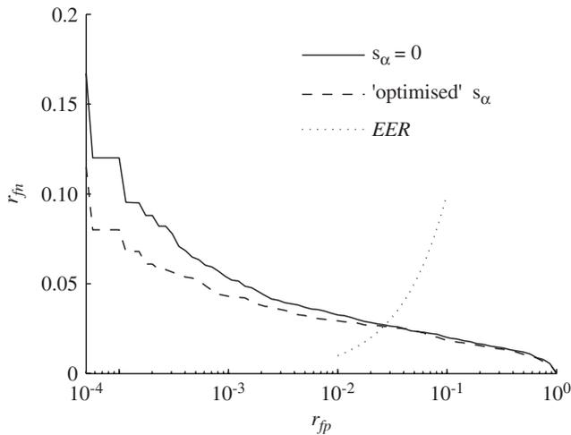
Fig. 6. Influence of the weighted inter-image differences.  $\overline{DET}$  curves for  $s_\alpha = 0$  and optimised  $s_\alpha$ . The equal error rate (EER) curve is also shown.
