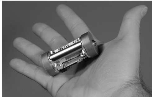
Fig. 1. Cy-mag 3D : ferromagnetic miniature climbing robot with cylindrical shape
