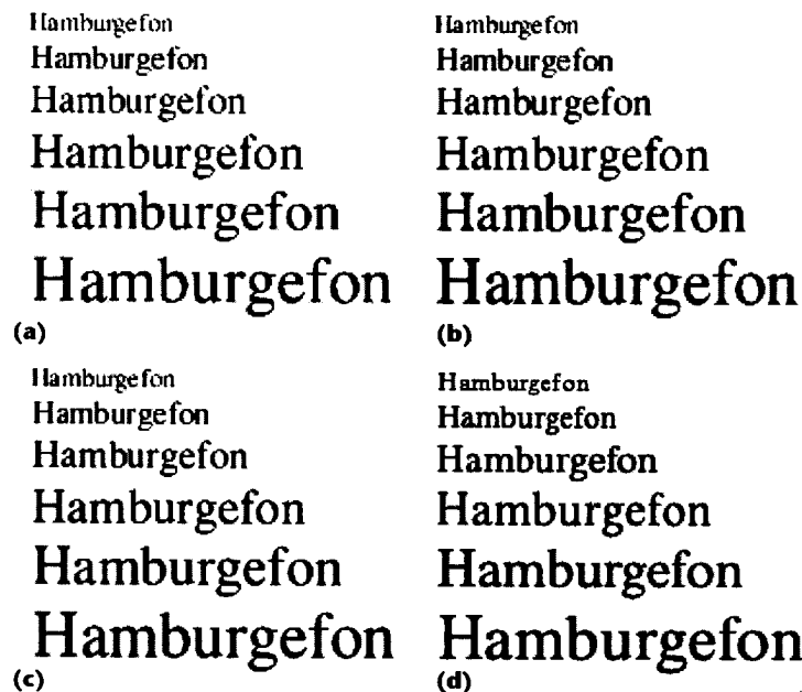
1 Filtered grayscale characters obtained by convolution with (a) a spline approximation of the sinc function, (b) a Hamming function, and (c) a rectangular function (box filter). These compare with (d) characters created manually pixel by pixel.
