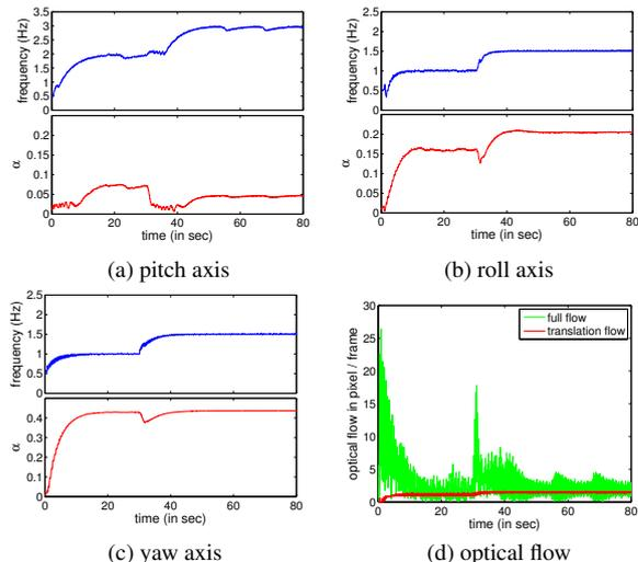
Fig. 1: Evolution of the frequency and the amplitude ( $\alpha$ ) of the oscillator when the salamander robot swimming. The frequency of swimming is initially 1Hz and at  $t = 30s$  the frequency is switched to 1.5Hz. Figure 1d shows the evolution of the mean optical flow magnitude over time as well as the flow due to the forward motion of the robot
