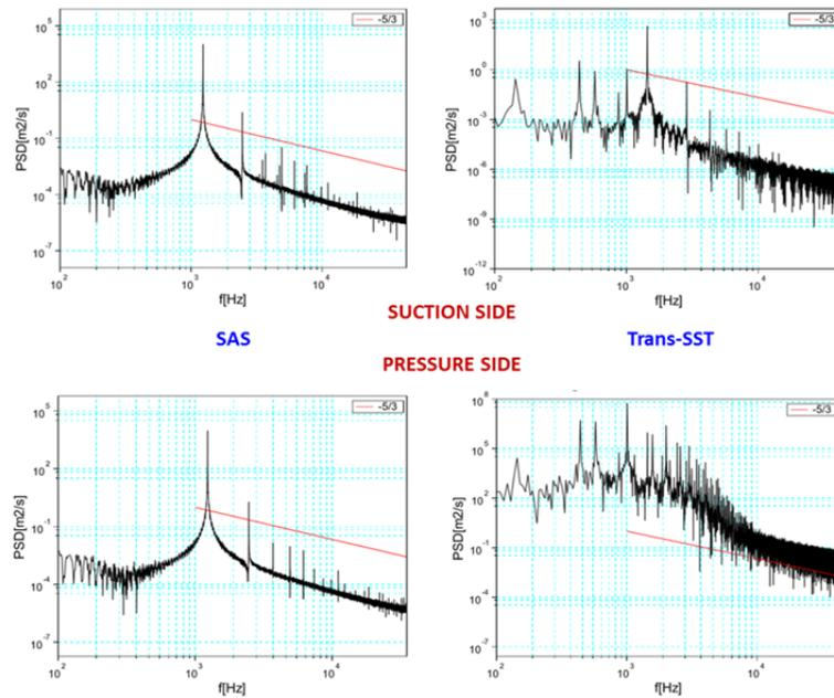
**Figure 4.** Power spectrum density analysis of the streamwise velocity fluctuation at the boundary layer outer sublayer at 50% of the hydrofoil chord.
