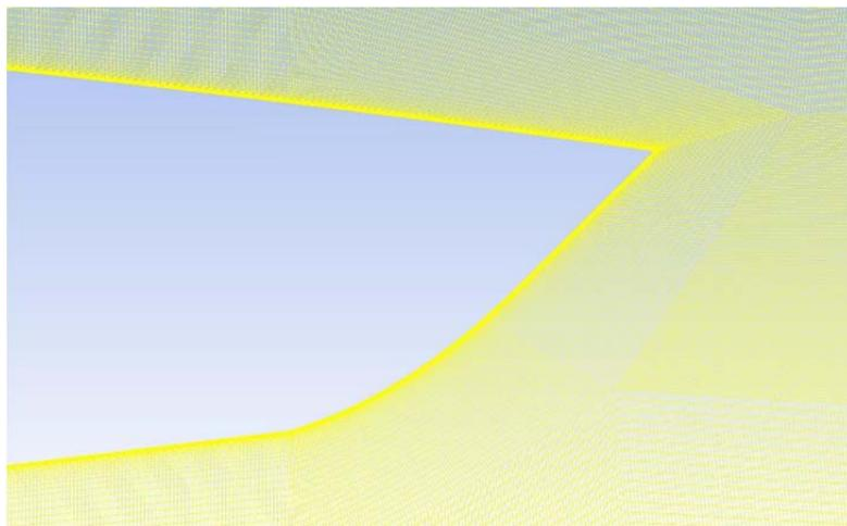
**Figure 1.** Trailing edge geometry and mesh detail for the Donaldson-type hydrofoil.
