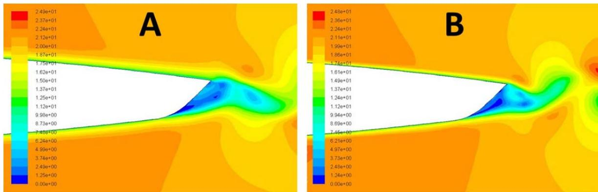
**Figure 3.** Velocity contours in the trailing edge of a Donaldson-type hydrofoil using (A) SAS and (B) Trans-SST turbulence models.
