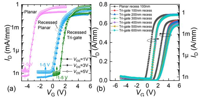
Fig. 3. (a) Comparison of the normally-off recessed tri-gate with planar and recessed devices under different  $V_{DS}$  (1V to 5V). (b) Comparison of planar recessed transistors with recessed tri-gate under different recess length (100nm to 600 nm).
