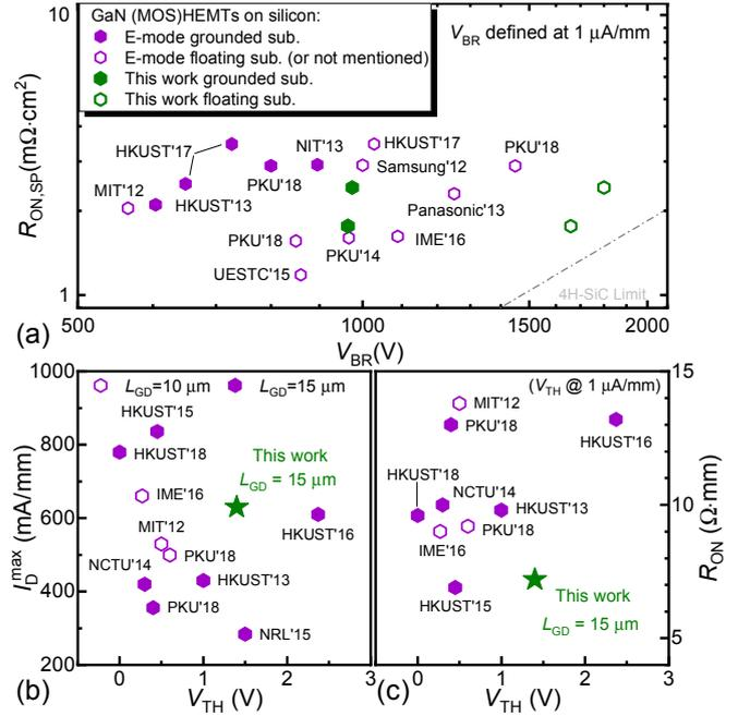
Fig. 7. Benchmarking of (a)  $R_{ON,SP}$  versus  $V_{BR}$  of the recessed tri-gate against E-mode GaN-on-Si transistors, by defining  $V_{BR}$  at  $I_{OFF} < 1 \mu A/mm$  with floating and grounded substrates. (b)  $I_D^{\max}$  and (c)  $R_{ON}$  versus  $V_{TH}$  (defined at 1  $\mu A/mm$ ). For fair comparison,  $L_{GD}$  smaller than 10  $\mu m$ , and literature results with unspecified  $R_{ON,SP}$  or  $I_{OFF}$  were not included.
