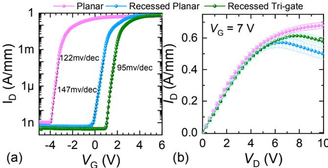
Fig. 2. Comparison of planar, recessed planar and recessed tri-gate devices. (a) Transfer at  $V_{DS} = 5$  V and (b) Output characters of the three device with  $V_G = 7$  V. The  $L_{GS}$ ,  $L_G$  and  $L_{GD}$  were 1.5, 2 and 15  $\mu\text{m}$ , respectively, and  $FF$  was 0.66.
