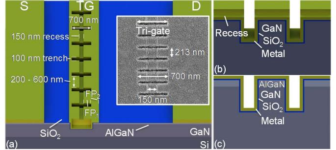
Fig. 1. (a) 3D schematic of recessed tri-gate MOSFET. Inset: zoomed SEM images of tri-gate regions. Cross-sectional views of recessed tri-gate MOSFET of (b) recessed regions and (c) tri-gate regions.
