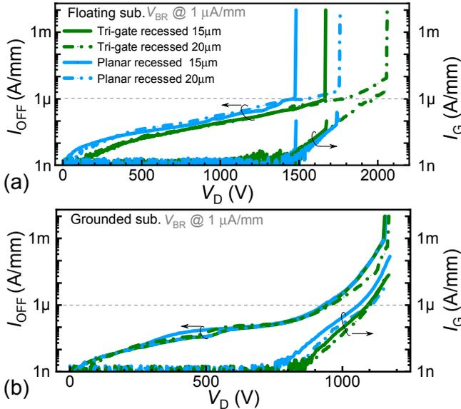
Fig. 6. Three terminal breakdown characteristics of recessed tri-gate ( $V_G = 0$  V) and recessed planar ( $V_G = -1$  V) MOSFETs with  $L_{GD} = 15 \mu m$  and  $20 \mu m$ , for (a) floating and (b) grounded substrate.
