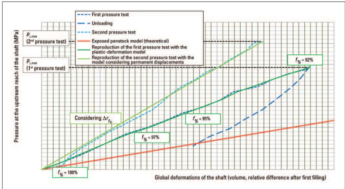
Fig. 4. Conceptual example of calibration of the model considering plastic deformations against pressure tests performed in the middle of the 20th century after the construction of an undisclosed high-head hydropower plant.
