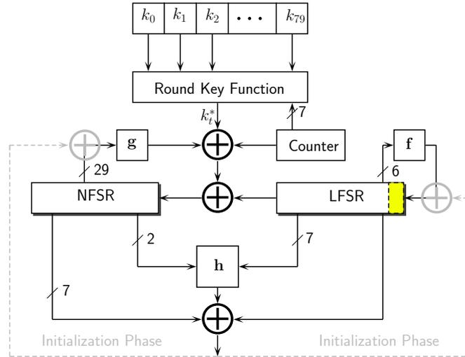
**Figure 1:** Block Diagram of Plantlet
