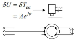
**Figure 5.** Forced response of an electrical system with torque excitation source  $\delta T_{ext}$ .
