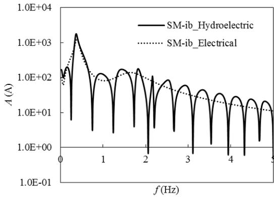
**Figure 11a.** Comparison of the forced response of the synchronous machine obtained with electrical and hydroelectric systems including PSS.
