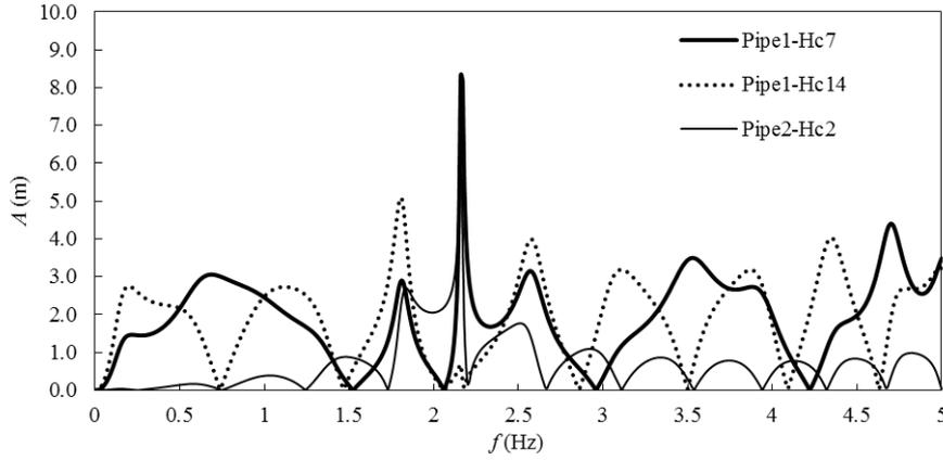
**Figure 9.** Forced response of the hydro-mechanical part
