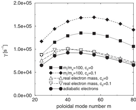
**Figure 7.** Growth rates of  $n = 2$  modes versus  $m$  calculated for different bumpiness parameters,  $c_0$  and ion to electron mass ratios, in a global simulation with both gyrokinetic ions and electrons, for W7-X-like parameters.
