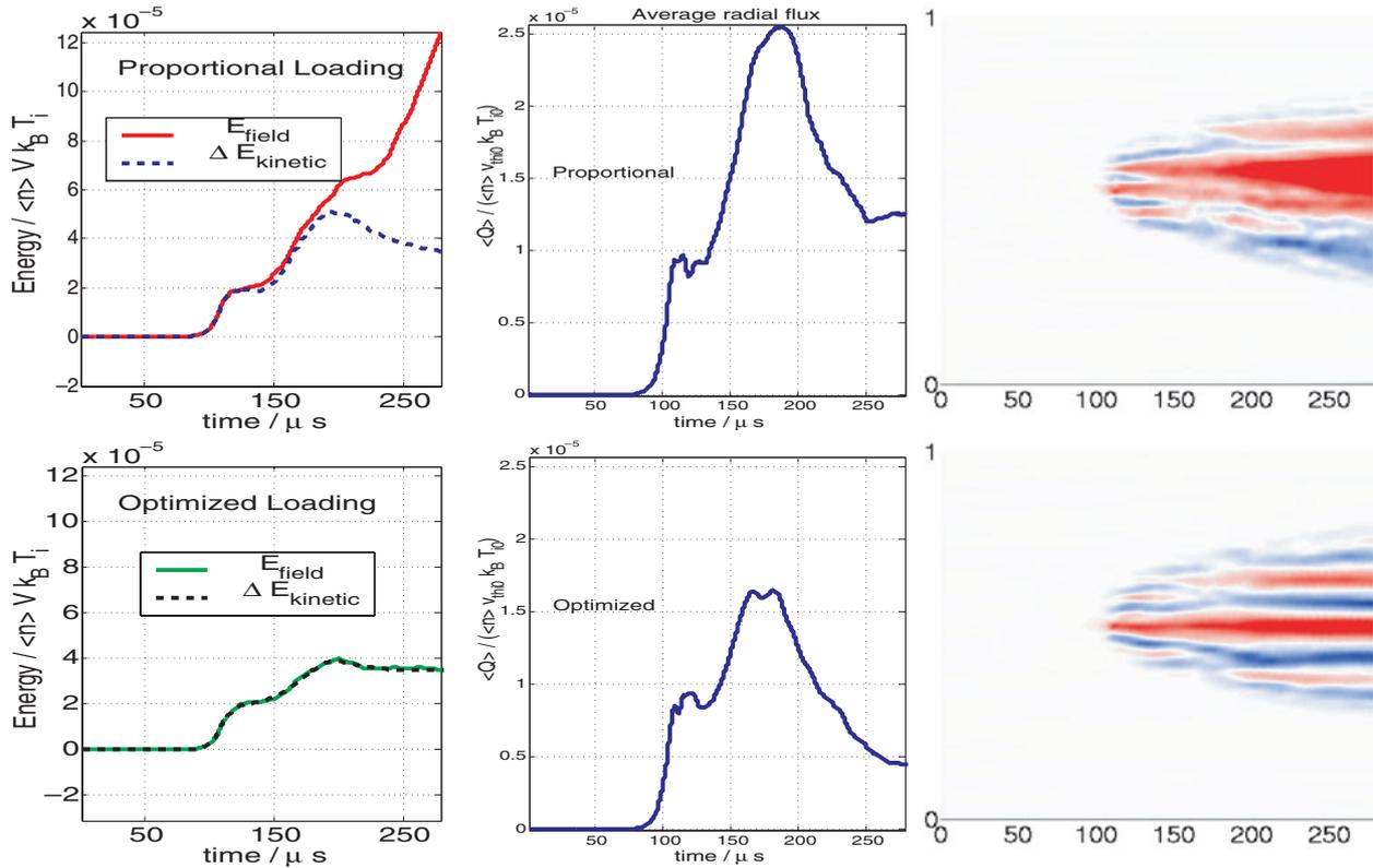
**Figure 1.** Field and kinetic energy (left), average radial heat flux (middle) and zonal  $E \times B$  component  $E_{r00}(r, t)$  (right, red for positive,  $\max = 24 \times 10^3 \text{ V m}^{-1}$ , blue for negative,  $\min = -24 \times 10^3 \text{ V m}^{-1}$ ) versus time, for an unoptimized (proportional) loading (top) and after loading optimization (bottom).
