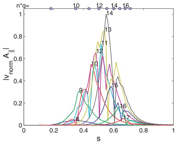
**Figure 8.** Left: growth rate of  $n = 7$  toroidal ITG and AITG modes versus  $\beta$ , normalized to  $\omega_{\text{norm}} = 3 \times 10^4 \text{ s}^{-1}$ . The critical  $\beta$  for ideal MHD ballooning is shown by the vertical line. Right: poloidal Fourier components of a  $n = 7$  toroidal AITG eigenmode at  $\beta = 6\%$  versus normalized minor radius,  $s = \rho/a$ , showing the resonant behaviour at rational  $q$  values, indicated by the circles on the top axis.
