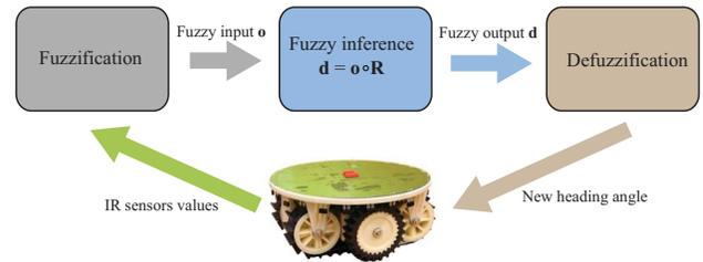
Fig. 7: The overview of the obstacle avoidance system.
