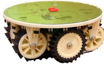
Fig. 2: The base module of the marXbot robot.
