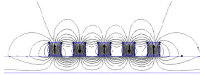
Figure 2: Simulation of magnets with a  $180^\circ$  shift at each increment.  $\delta x_k$  is the space between two magnets.
