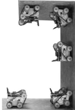
Figure 5: The robot moving from floor to ceiling
