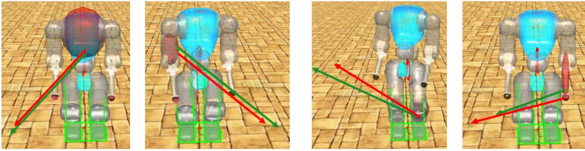
**Figure 1:** Snapshots of force estimation performance for a 30kg robot performing squatting and yaw motions. Forces are about 10N applied in different directions to various links on the robot. Red arrows show the actual force while green arrows show the estimation. The associated body link is also shown by the approximate red ellipsoid.
