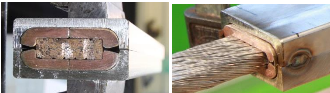
Fig. 2. Conductor assembly with the half-size profile (left) and full-size profile (right) mixed matrix stabilizer.
