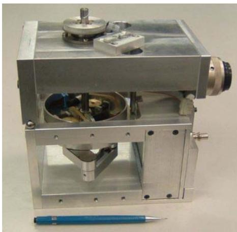
Fig. 5: The 4 DOF robot associated with a microbox
