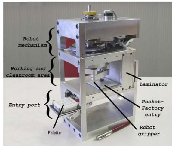
Fig. 3: The microbox is a module of the Pocket-Factory
