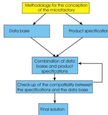
Fig. 11: Flow chart for the methodology of conception for the microfactory
