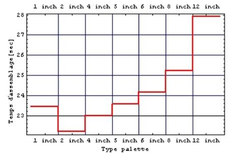
Fig. 10: Assembly time as function of the size of the palettes.
