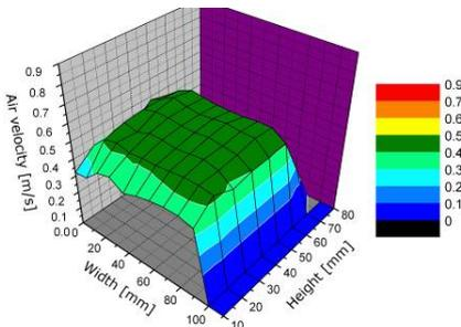
Fig. 8: Air velocity measured 15mm after the laminator
