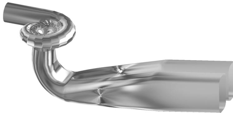
Fig. 2: Computing domain of the GMS Unit 2 Francis turbine
