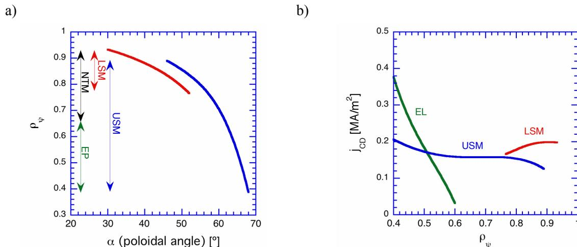
Figure 2 (a) Extension of the total access range ( $\rho_\psi=0.4$  to  $0.93$ ) of the upper (USM) and lower (LSM) steering mirrors from the zone of NTMs ( $\rho_\psi=0.64$  to  $0.93$ ) by partial overlapping of the two steering mirrors access ranges. (b) Comparison of  $j_{CD}$  between either the two steering mirrors of the UL with 13.3MW and the EL launcher (EL) with 20MW.
