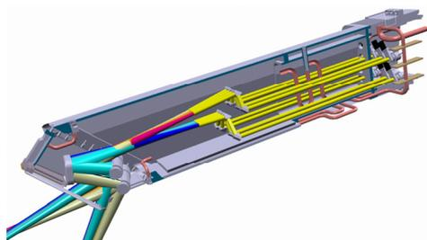
Figure 1: a) The ITER ECH upper launcher shown in a port plug and b) the range of  $q=2$  and  $3/2$  flux surfaces that the UL is required to access for NTM stabilisation.
