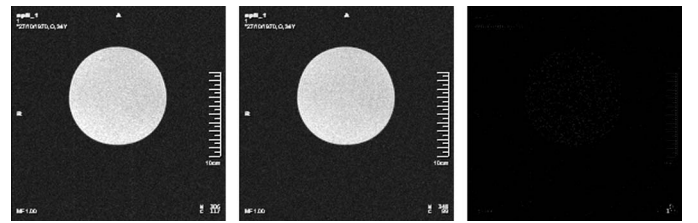
Fig. 13. Functional images of the cylindrical phantom when the robot was not inside the shielded room (left) and when the motor was in motion at the entry of the scanner bore (center). The subtraction of these images shows no shift (right).
