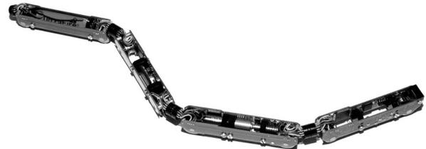
Fig. 1. View of the complete robot *Tubulo*, using magnetic wheels.
