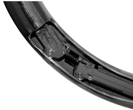
Fig. 8. Robot passing a curve going up.
