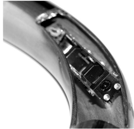
Fig. 9. Robot stuck in a lateral curve.
