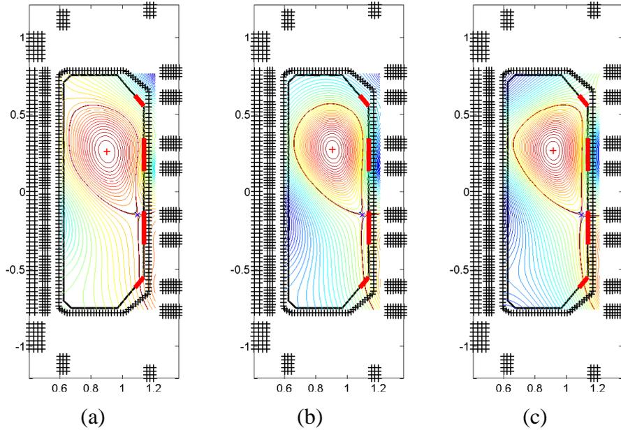
Figure 2. Poloidal flux level lines for free boundary equilibria in TCV tokamak calculated with the SPIDER code. Plasma elongation  $\kappa \sim 1.6$ . Upper triangularities (a) 0.3, (b) 0.0, (c)  $-0.4$ . The positions of full toroidal coverage zones with graphite tiles are shown by thick red lines.
