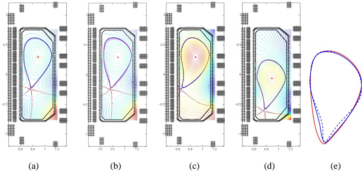
Figure 4. Poloidal flux level lines for free boundary snowflake equilibria: (a) fit to the shot #36151 boundary  $\delta_{up} = 0.2$ , (b) increased upper triangularity  $\delta_{up} = 0.4$ , (c) large snowflake point triangularity  $\delta_{down} = 0.8$ , (d) snowflake on the floor of the TCV vacuum vessel; (e) snowflake boundary from Fig.4b (blue) compared to the X-point boundary (red) and to the snowflake boundary with large pedestal current density (dashed).
