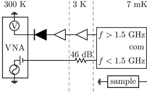
Fig. 3. Experimental setup. Diode symbol represents a power detector. VNA=Vector Network Analyser
