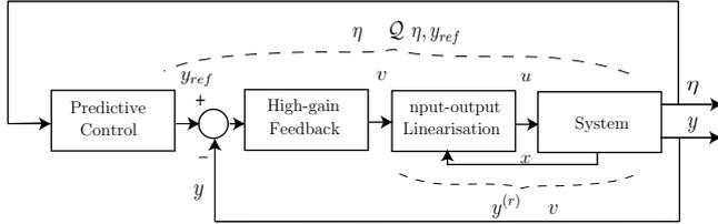
**Figure 1:** Cascade control scheme
