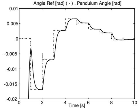
**Figure 3:**  $\theta_{ref}$  and  $\theta$  in the cascade control scheme
