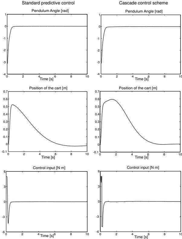
**Figure 2:** Standard predictive control of an inverted pendulum on a cart
