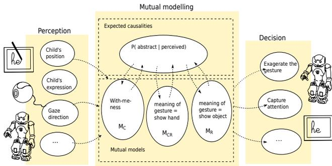
Fig. 1. **Overview of the cognitive architecture.** Yellow squares represent the main parts. White ellipses represent modules. It shows possible devices used for perception and decisions with the context of the CoWriter Activity. We illustrate the architecture with a situation of misunderstanding : the child has a bad interpretation of the gesture of the robot. In order to resolve this misunderstanding, a possible decision could be to exaggerate the movement.
