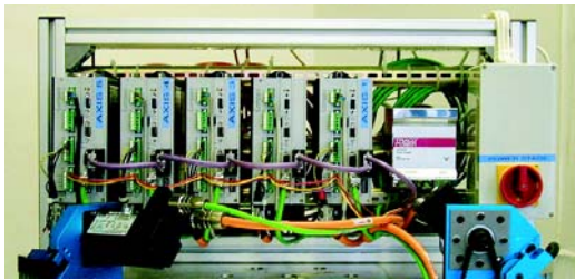
Figure 5: The Control Hardware. The figure shows the 5 drives of our prototype. They contain the PROFIBUS-interface, the control-"intelligence" and the amplifiers.
