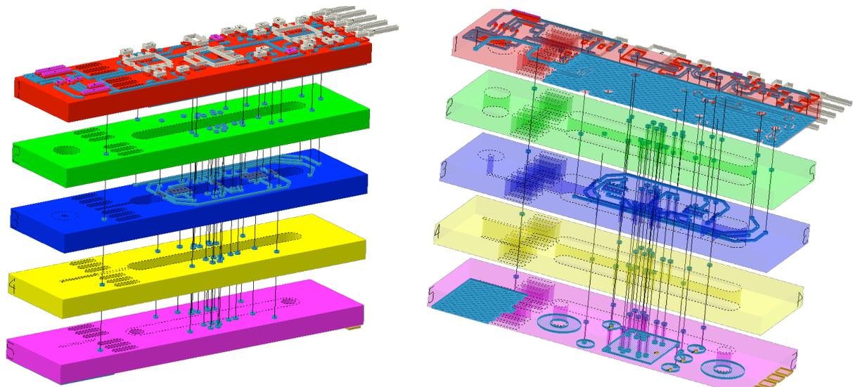
Fig. 4. (a) 3D exploded top view of the integrated sensor, showing the five LTCC tapes. (b) 3D exploded bottom view, semi-transparent.
