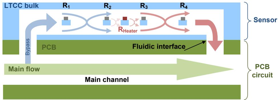
Fig. 3. Schematic view of the flow sensor demonstrator<sup>2</sup> mounted on a fluidic PCB, depicting the bypass and thermistors.
