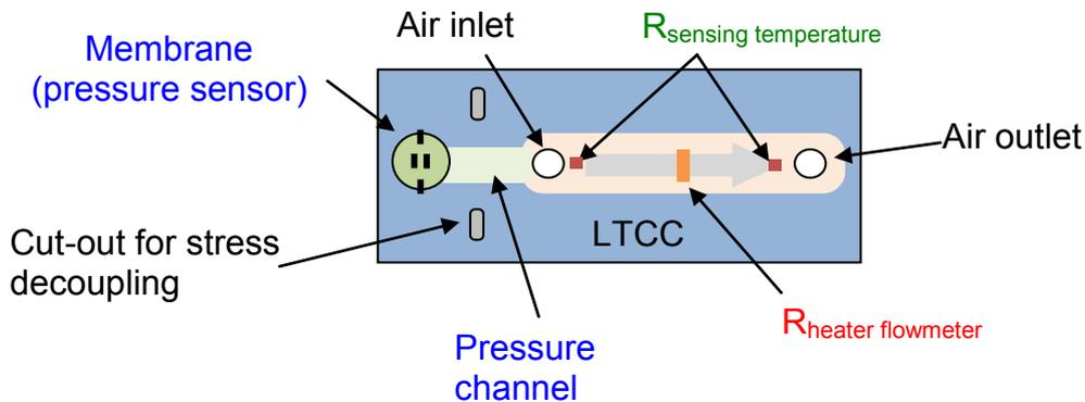
Fig. 2. Schematic top view of the integrated sensor, showing the placement of the fluidic functions and the elongated shape of the circuit.
