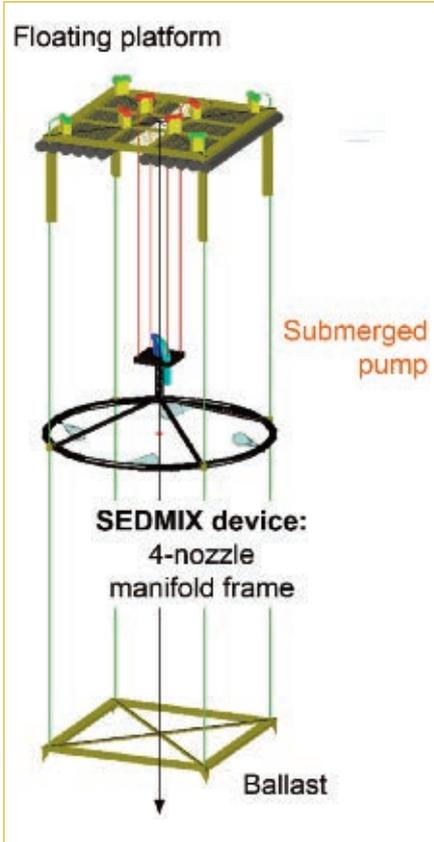
Figure 5. Schematic drawing of the SEDMIX device with a floating platform and a ballast anchor structure on the reservoir bottom
