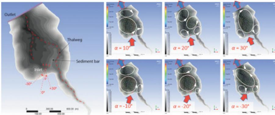
Figure 3. Bed topography and velocity vectors at the water surface for the flow discharge of 90 m<sup>3</sup>/s considering seven alternative water release (flow into the reservoir, red arrow) angles  $\alpha$  varying from +30° to -30° [4]. The power intake is located at the dam location (blue arrow, see also Figure 1)
