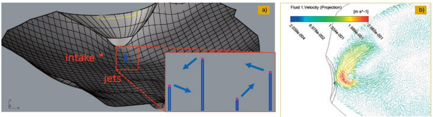
Figure 6. a) Water intake and SEDMIX jet location in the numerical model of the Trift Reservoir in the Swiss Alps, the jets discharge horizontally; and b) induced flow field on the horizontal jet plane
