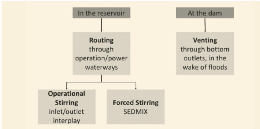
Figure 2. Innovative solutions for fine sediment management in seasonal reservoirs developed at EPFL
