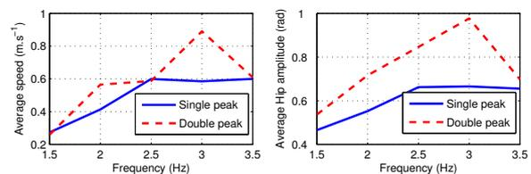
Fig. 3 Amplitude and speed average comparison for two different knee joint control strategies.
