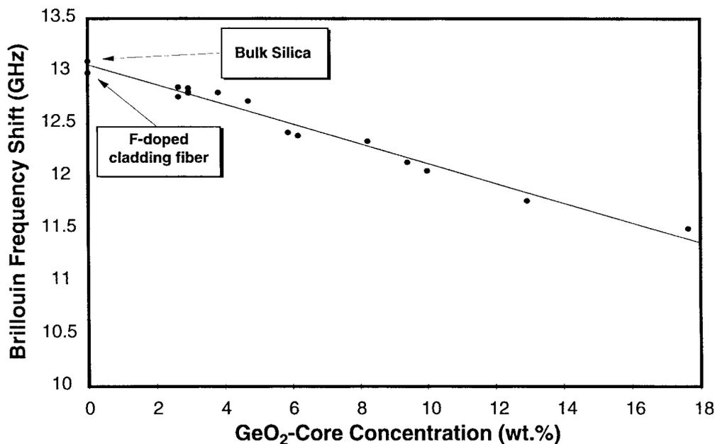
Fig. 7. Measured dependence of the Stokes frequency shift  $\nu_B$  on the GeO<sub>2</sub>-core concentration.
