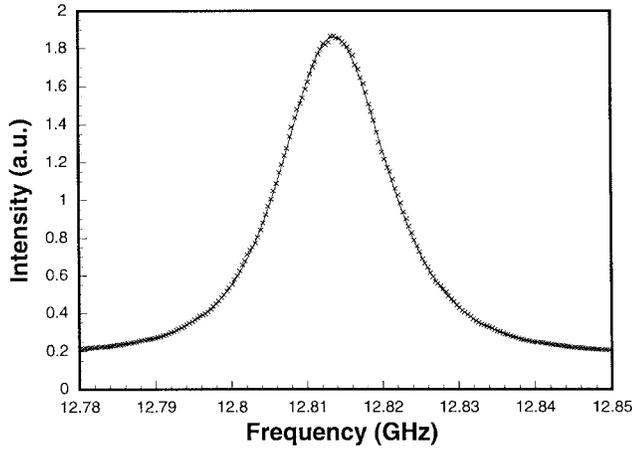
Fig. 4. Brillouin gain spectrum of a 700-m single mode fiber. The experimental data (crosses) perfectly fit the hyperbolic cosine of a Lorentzian function.  $\Delta\nu_B = 35.8$  MHz,  $\nu_B = 12.8138$  GHz.
