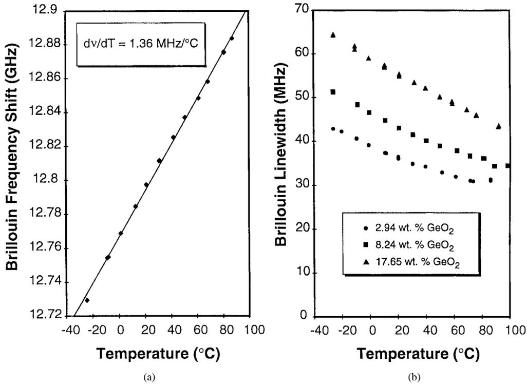
Fig. 10. Central frequency (a) and linewidth (b) of the Brillouin gain spectrum as a function of temperature. Linewidth measurements are shown for fibers with different GeO<sub>2</sub>-core content.
