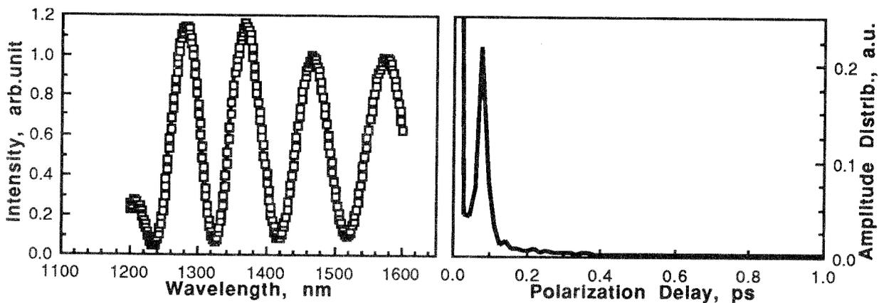
Fig.4 Detected intensity at the interferometric loop output for a 3-m sample of standard single-mode fibre showing no polarization fluctuation, and corresponding Fourier transform which reduces to a single peak in this case.
