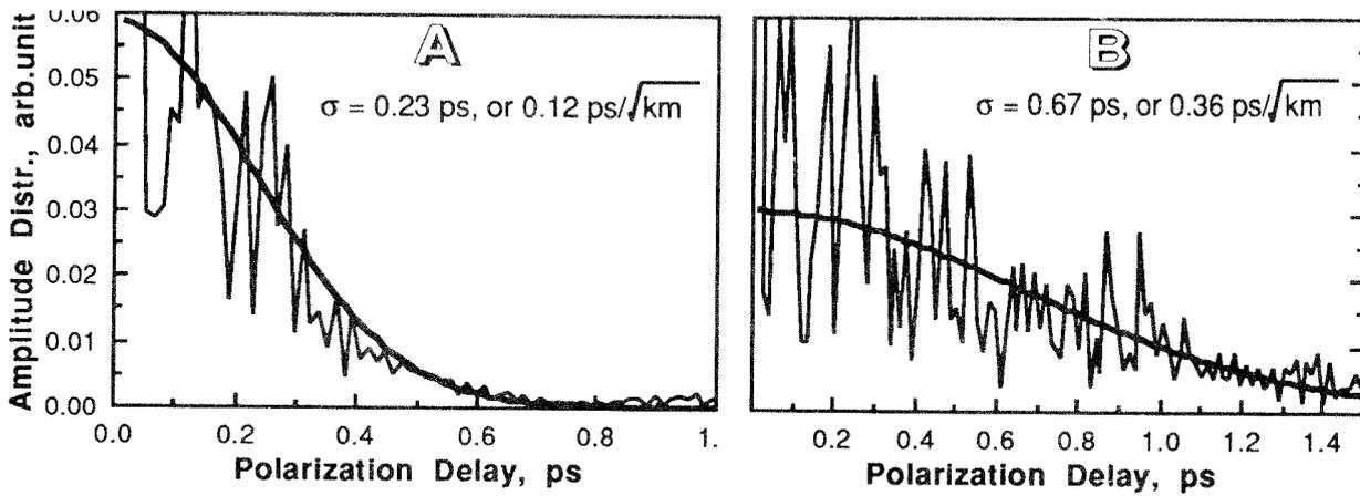
Fig.3 Fourier transform of the detected intensities shown in Fig.2, representing the distribution of polarization delay, and corresponding Gaussian fit with its standard deviation.
