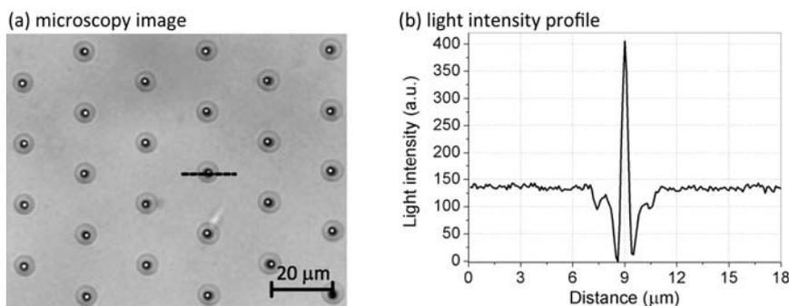
Figure 3: (a) Microscopic image obtained from a  $32\times$  objective ( $NA = 0.4$ ) objective, which focuses onto the microsphere focal plane. The light intensity along the dashed line in (a) is shown in (b). The intensity within the photonic nanojet is about 3 times the background.
