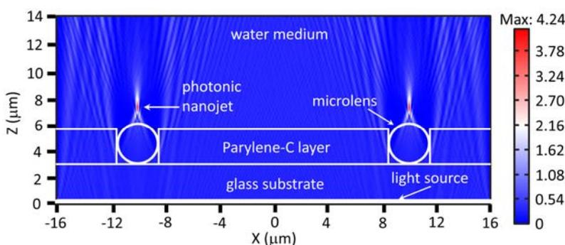
Figure 4: FEM simulation (Comsol Multiphysics) of the light propagating through the glass substrate, the Parylene-C layer and two dielectric microspheres, which are immersed in water medium. The microspheres are used as microlenses to focus the illumination light coming from below the glass substrate.
