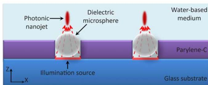
Figure 1: Schematic illustration of the microlens array, generated by patterning dielectric microspheres into a microwell array, the latter being fabricated in a Parylene-C layer on a glass substrate. Due to their high refractive index, the microlenses can be used in a water-based medium. When the microsphere is illuminated by a light source from below, it focuses the light into a small region, also named ‘photonic nanojet’.
