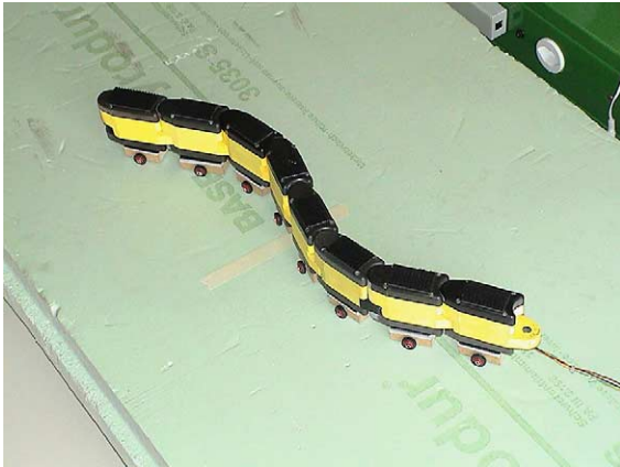
Fig. 4. The robot (here with passive wheels) in the experimental setup.
