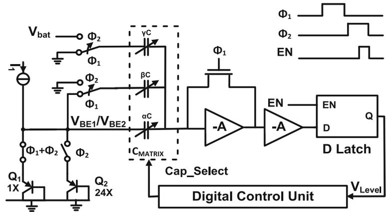
When  $V_{bat}$  reaches to the  $V_{EOD}$  limit, the SIC and the wireless transceiver are deactivated temporarily to avoid overdischarge.
