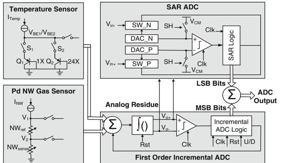
**Fig. 5** Circuit diagram of the first order incremental ADC
