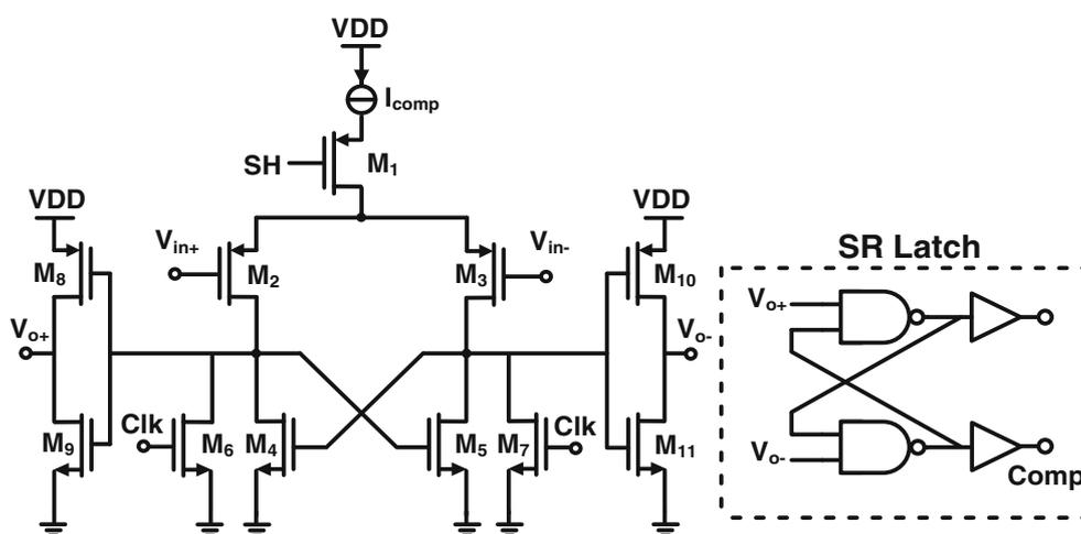
**Fig. 7** Circuit diagram of the latched comparator
