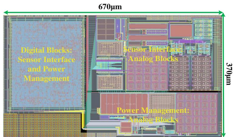
have been specified separately in this layout. Highly resistive poly resistors have been used as embedded resistors in the beta multiplier current source and oscillator. As these embedded resistors are sensitive to process variations, they are trimmed initially.
