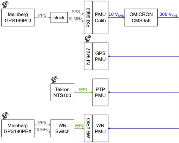
Fig. 3. Measurement setup for the assessment of the PMUs' phase estimation accuracy. The PMU calibrator generates the user-defined test waveforms, that are amplified up to 300 V by the CMS 356 OMICRON amplifier, and then supplied to the three considered PMUs, relying on GPS, PTP and WR time dissemination, respectively.
