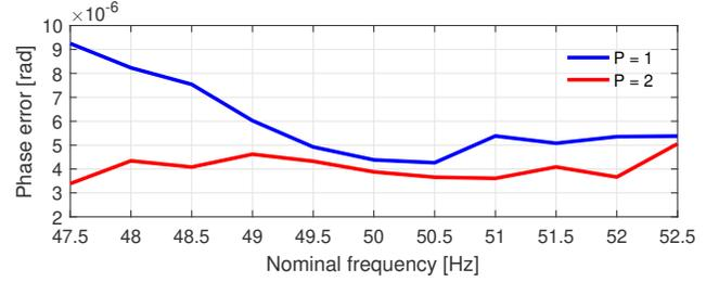
Fig. 2. Phase estimation error as provided by e-IPDFT as function of the fundamental frequency, when the iteration number  $P$  of the compensation routine is set equal to 1 (blue) and 2 (red), respectively. The additive white Gaussian noise produces a signal-to-noise ratio of 85 dB.
