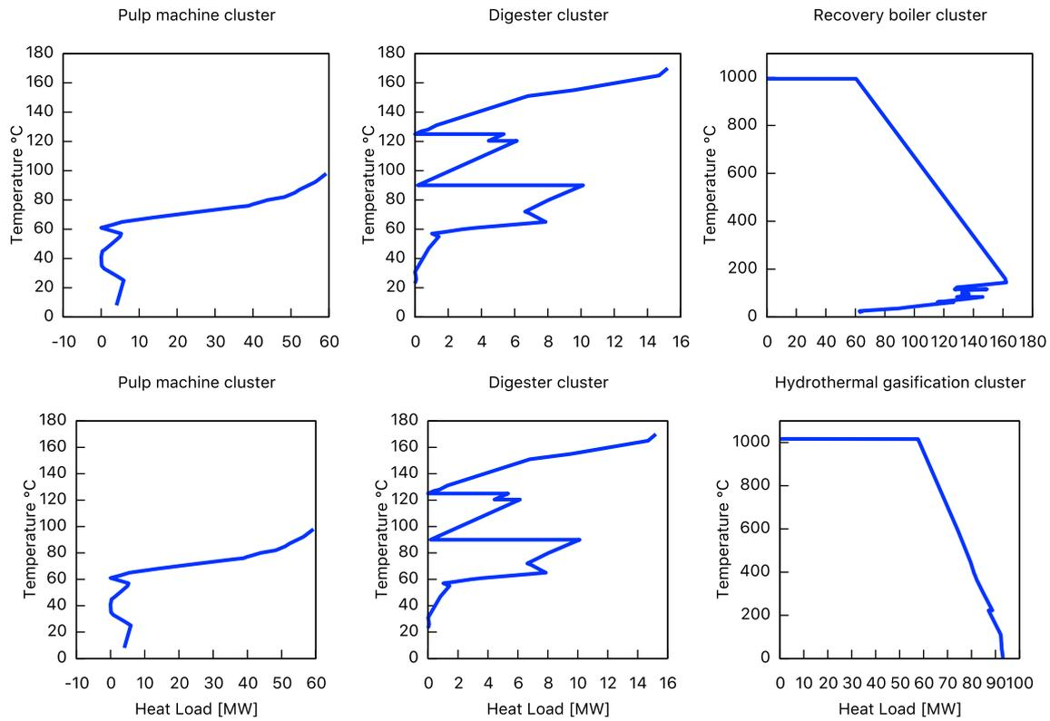
**Figure 3:** Grand composite curve of MER of conventional Kraft mill and hydrothermal gasification
