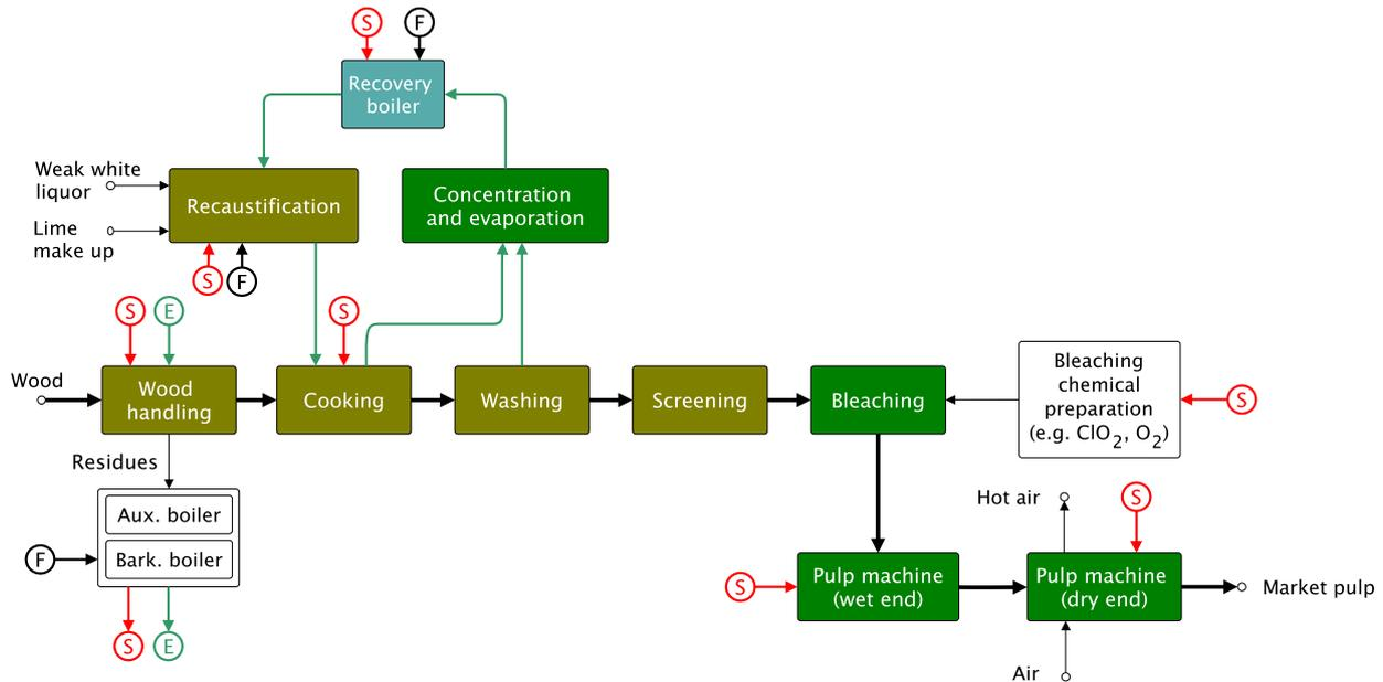
**Figure 1:** Block flow diagram of a generic Kraft process, adapted from [13]
