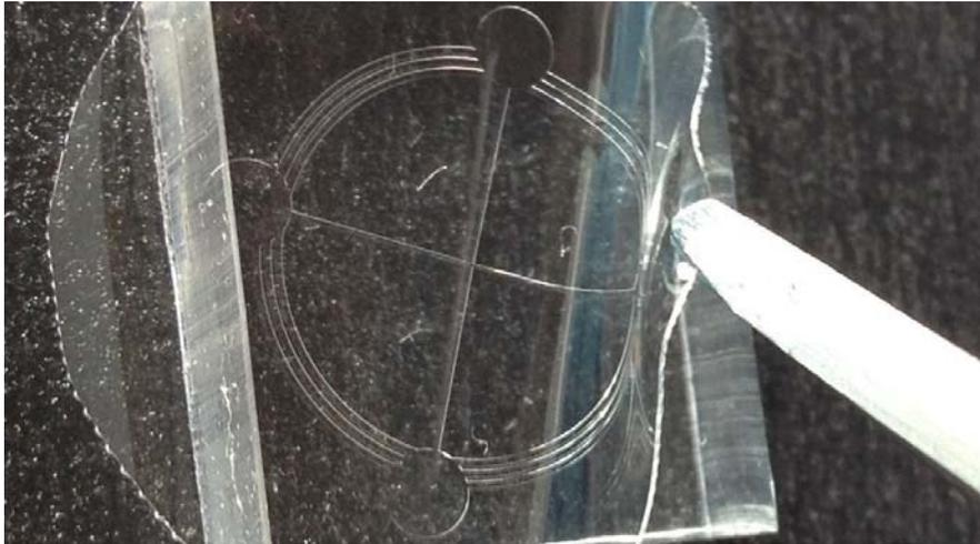
**SI Figure 2.** Photograph of the transverse plane microfluidics formed in a thin PDMS layer. The layer is transferred to a thicker one for punching process defining the trap chamber.
