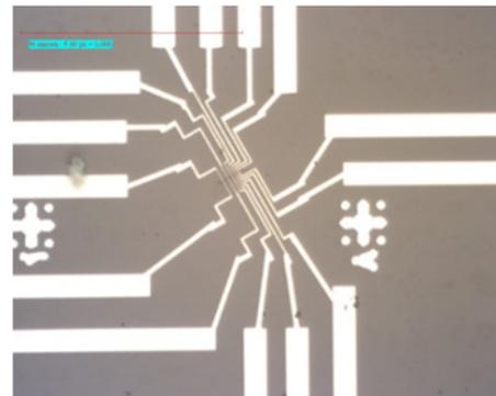
Fig. 1. An optical image of an InAs nanowire chip.
