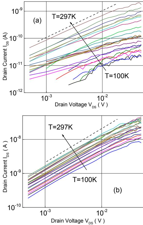
Fig. 2.  $I_D(V_{DS})$  dependences of the sample with  $L = 3 \mu\text{m}$  at two gate voltages (a)  $V_G = 0$  and (b)  $V_G = 2 \text{ V}$  as well as at different temperatures in the range from  $T = 100 \text{ K}$  to  $T = 297 \text{ K}$ . The change step is  $\Delta V_{DS} = 0.5 \text{ mV}$ . The curves are smoothed by the Savitzky-Golay method, a second-order polynomial, and the window length is 15 points. The dashed line indicates a linear relationship.
