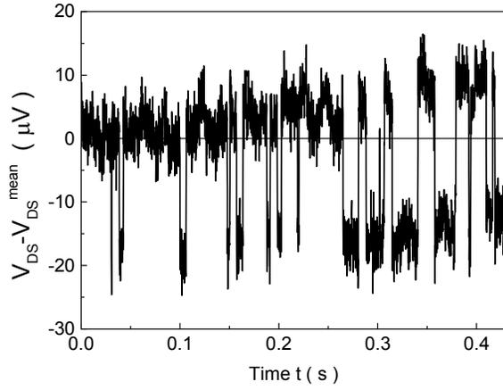
Fig. 4. Time trace demonstrating RTS behavior in the drain current of an NW sample ( $L = 3 \mu\text{m}$ ),  $V_{DS} = 20 \text{ mV}$ ,  $V_G = 0$ ,  $T = 220 \text{ K}$ .
