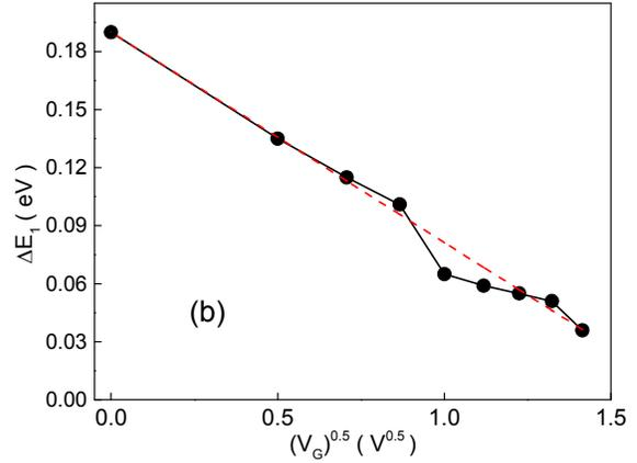
Fig. 5. (a) Temperature dependences of the conductivity of InAs NW with a length of  $L = 3 \mu\text{m}$  at  $V_G = 0$  and several voltages of  $V_{DS}$  (indicated in the inset). (b) The dependence of the activation energy  $\Delta E$  as a function of  $\sqrt{V_G}$ , obtained for  $V_{DS} = 50 \text{ mV}$ . The dashed line indicates the calculated dependence obtained in accordance with Eq. (1).
