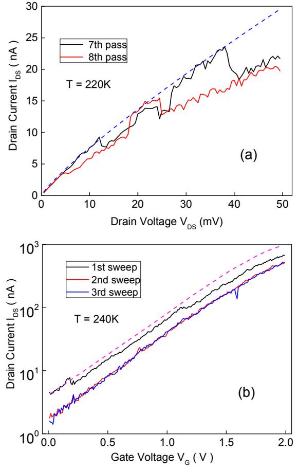
Fig. 3. Typical current-voltage (a) ( $V_G = 1.75 \text{ V}$ ) and drain-gate (b) ( $V_{DS} = 25 \text{ mV}$ ) characteristics of an InAs NW sample with length  $L = 3 \mu\text{m}$ , measured successively with a period of (a) 6 s and (b) 12 s. The dashed lines show the estimated curves in the absence of a current change. The measurement temperature is shown in the figure.
