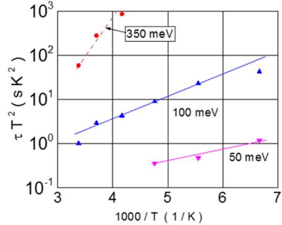
Fig. 6. Arrhenius plot obtained using noise spectra measured at different temperatures for the sample with  $L = 1200 \text{ nm}$ .
