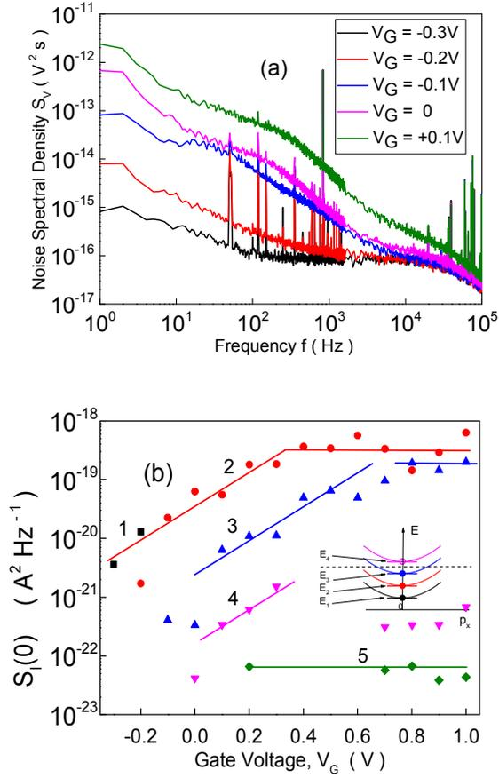
Fig. 7. (a) Noise spectrum of sample 5 ( $L = 600$  nm),  $V_{DS} = 10$  mV,  $V_G = -0.3$  V to  $+0.1$  V,  $T = 150$  K; (b) the low-frequency Lorentzian noise plateau values,  $S_l(0)$ , extracted from measured noise spectra, as a function of gate voltage,  $T = 300$  K. The inset shows a schematic of the band structure with quantum levels of 1D conductivity in an NW structure.
