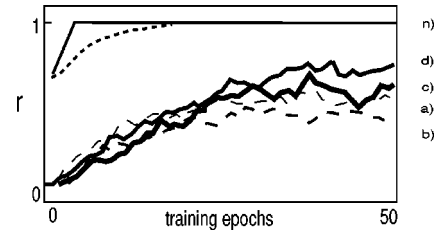
FIG. 2. Transient behavior of the recognition rate r when images are associated with random output vectors of length m=40 . Curves a-d : artificial images, gliding averages for \lambda=0.2 . Noise combinations (\sigma_l^2, \sigma_r^2) as follows: a , (0, 0) ; b , (0, 0.05) ; c , (0.1, 0.05) ; d , (0.1, 0) . Curve n : natural images, where noise is added only during recall ( \sigma_r^2=0.05 ). Dashed curve: gliding average for \lambda=0.2 .
