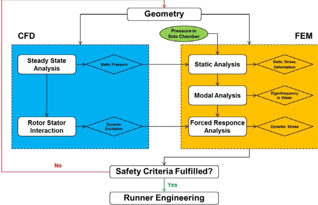
Figure 1. Runner safety check procedure
