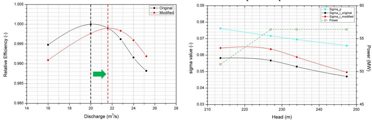
**Figure 8.** Impact of modification on efficiency (left, relative efficiency over discharge, peak position shifted to right side) and cavitation (right, sigma incipient lower than sigma plant indicates cavitation free)
