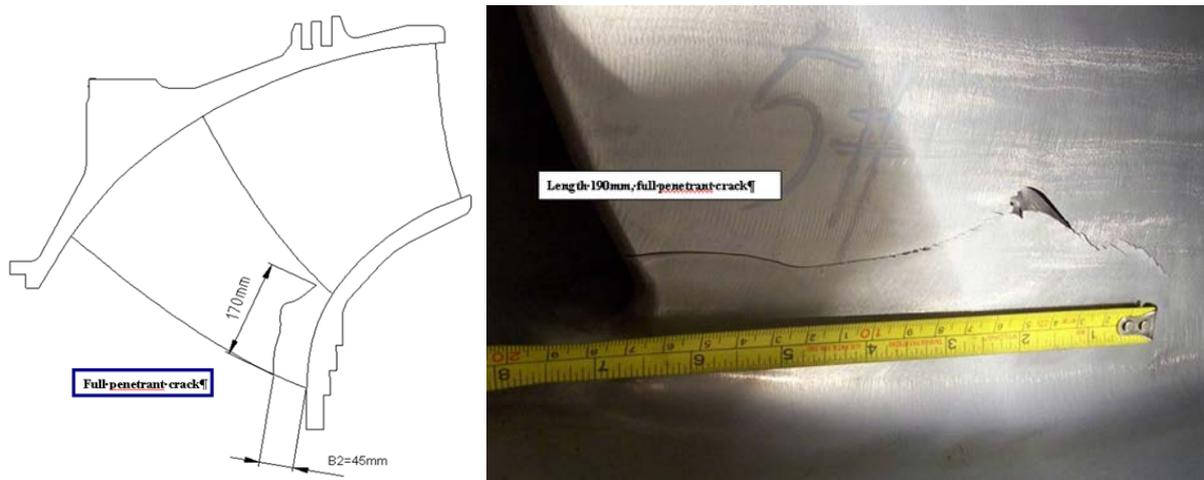
**Figure 2.** Crack observed on the long blade close to runner band
