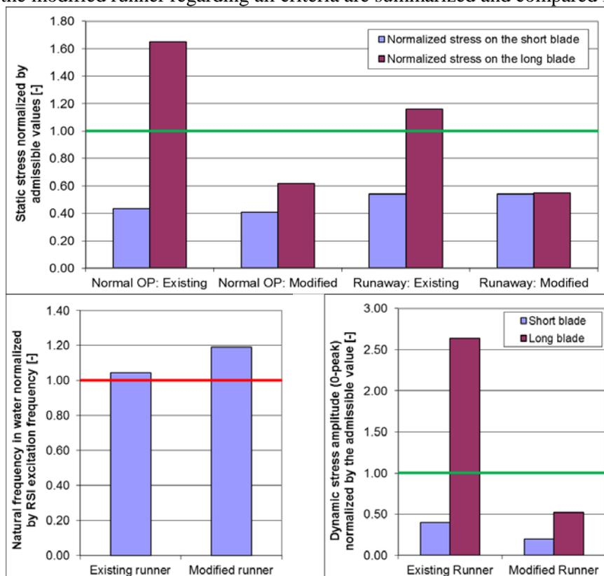
**Figure 7.** Effect of modification on trailing edge, in terms of maximum static stress (top, normalized by admissible values depending on operating conditions), natural frequency (down left, normalized by RSI excitation frequency) and maximum dynamic stress amplitude (down right, normalized by admissible value)
