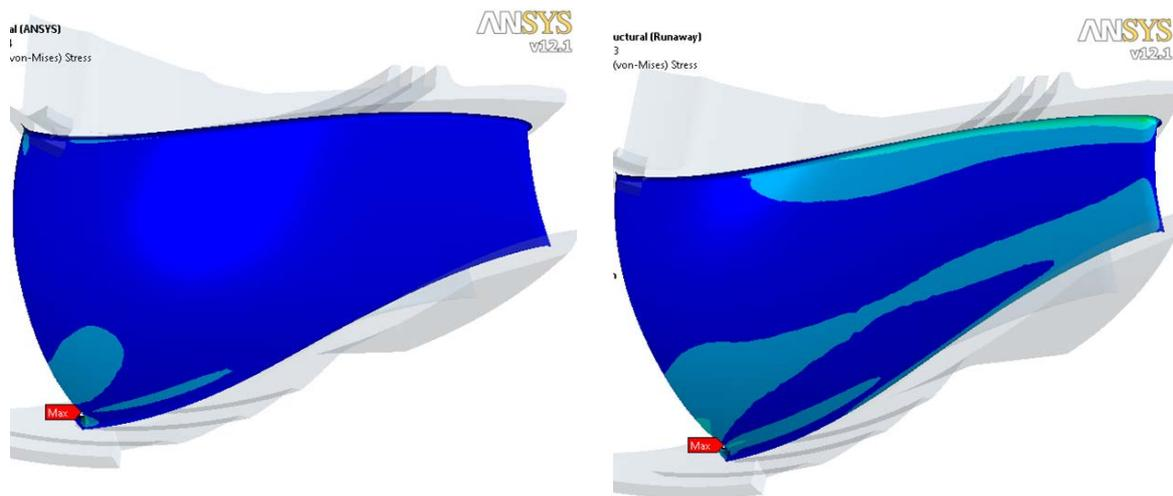
**Figure 3.** Distribution of static stress on long blade at normal operation point (left) and runaway point (right), location of maximum stress coincide with the crack start point. Please note that the scales of the colour schemes in these 2 pictures are different.
