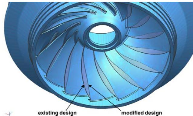
**Figure 6.** Comparison of existing runner and modified runner
