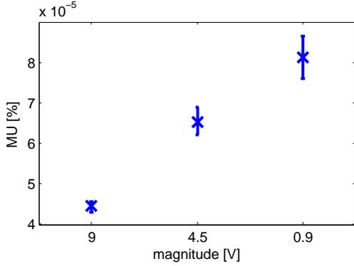
Fig. 6. Normalized magnitude uncertainty as function of the fundamental amplitude. It should be noticed that MU keeps below  $1 \cdot 10^{-4}\%$ , even when  $A$  is decreased up to 10% of the nominal value.
