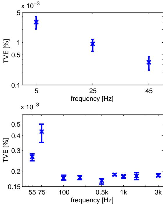
Fig. 12. TVE as function of frequency in the range provided for harmonic and interharmonic components, i.e. from 5 to 25 Hz (top) and from 75 to 3000 Hz (bottom).
