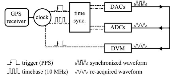
Fig. 4. Measurement setup for the assessment of magnitude uncertainty. The generated waveforms are simultaneously sent to the ADC stage and to the digital multimeter (DVM). The synchronization between the two measurement chains is guaranteed by the same trigger provided by the atomic clock.
