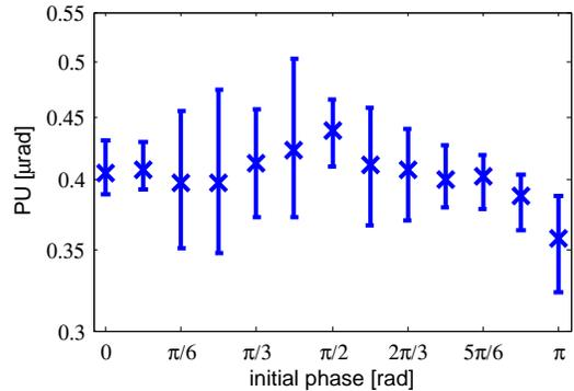
Fig. 9. Phase uncertainty as function of the fundamental initial phase. In the entire considered range, PU does not exhibit significant variations, between  $0.35$  and  $0.5 \mu\text{rad}$ .
