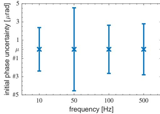
Fig. 18. Initial phase uncertainty due to DAC initial phase contribution as function of sPPS and s frequency.
