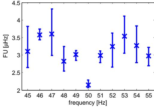
Fig. 10. Frequency uncertainty as function of the fundamental frequency. A rather symmetric trend is noticed as the fundamental frequency deviates from its nominal value,  $f = 50$  Hz. In the worst case, FU does not exceed  $4.5 \mu\text{Hz}$ .
