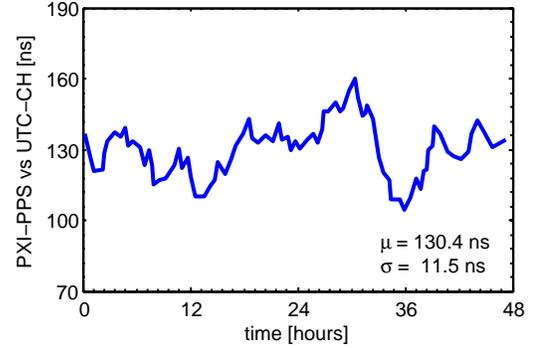
Fig. 13. Time deviation between the PPS signal provided to the PXI (PXi-PPS) and the PPS signal directly derived from UTC-CH (UTC-CH). Over an observation interval of two days, the standard deviation is lower than 12 ns, corresponding to a phase uncertainty of  $4 \mu\text{rad}$  at 50 Hz.
