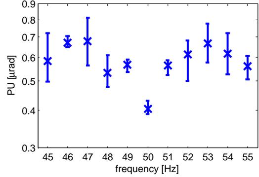
Fig. 8. Phase uncertainty as function of the fundamental frequency. A performance degradation is noticed as the fundamental frequency deviates from its nominal value,  $f = 50$  Hz. Nevertheless, in the worst case, PU does not exceed  $0.85 \mu\text{rad}$ .
