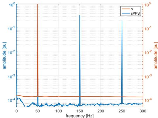
Fig. 17. Detail for the DFT module of the signals sPPS (blue) and s (red), expressed in pu. Nevertheless, the adopted frequency resolution allows for minimizing spectral leakage effects.
