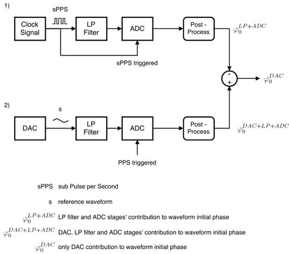
Fig. 15. Initial phase displacement due to imprecise synchronization between generation and acquisition stage. In 1, we evaluate the uncertainty due to low-pass filter and acquisition stages. In 2, we determine the uncertainty due also to generation stage. The subtraction provides the single DAC contribution.
