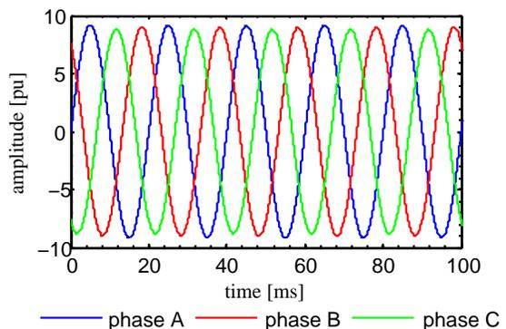
Fig. 19. Detail of three-phase unbalanced waveform, compliant with the limits provided by EN 50160. Inverse and homopolar sequence energy correspond to nearly 2 and 0.0003% of the direct sequence energy, respectively.
