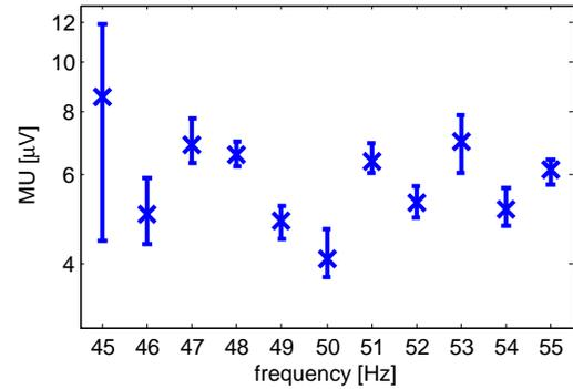
Fig. 5. Magnitude uncertainty as function of the fundamental frequency. MU tends to increase as the fundamental frequency decreases. The maximum value is obtained for  $f = 45$  Hz, when MU does not exceed  $12 \mu\text{V}$ .
