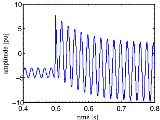
Fig. 20. Detail of a current in-rush event, as reproduced by the proposed PMU calibrator.
