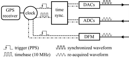
Fig. 7. Measurement setup for the assessment of frequency uncertainty. The generated waveforms are simultaneously sent to the ADC stage and to the counter (DFM). The synchronization between the two measurement chains is guaranteed by the same trigger provided by the atomic clock.
