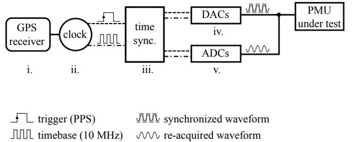
Fig. 1. Hardware architecture of the proposed validation system. Generation (DACs) and acquisition (ADCs) boards are aligned to UTC through the same synchronization board, that is disciplined by a GPS-receiver and a Rubidium atomic clock in order to enhance the stability of the internal time-base.
