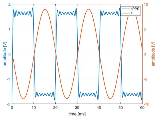
Fig. 16. Detail of the signals sPPS (blue) and s (red), as acquired in the upper and lower scheme of the routine for initial phase characterization. The difference between the corresponding initial phases accounts for the internal synchronization delay between generation and acquisition stages.
