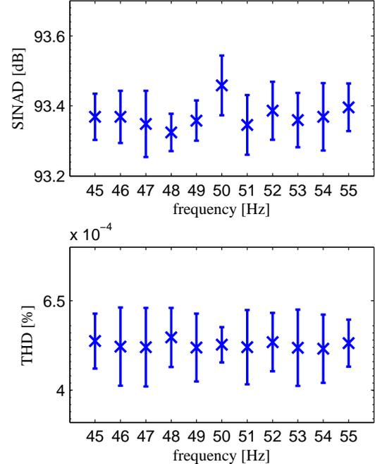
Fig. 2. Power quality assessment of the generated test waveform in terms of SINAD (top) and THD (bottom) in steady-state test conditions, as function of the fundamental frequency. The cross represents the mean value, whereas the bold line determines a confidence interval of three standard deviations.
