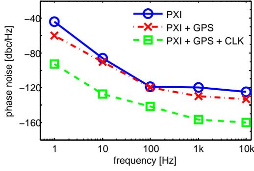
Fig. 14. Phase noise obtained with three different configurations: free-running PXI (circles), PXI disciplined by GPS receiver only (crosses), PXI disciplined by atomic clock and GPS receiver (squares). The last one guarantees a significant phase noise reduction over the considered frequency range.
