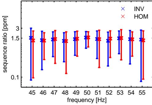
Fig. 3. Energy ratio of inverse (blue) and homopolar (red) sequence with respect to direct sequence, in steady-state test conditions, as function of the fundamental frequency. The cross represents the mean value, whereas the bold line determines a confidence interval of three standard deviations.
