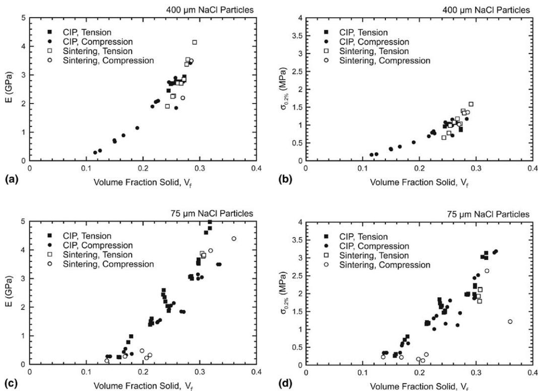
Fig. 4. The Young's modulus (graphs (a) and (c)) and 0.2% yield stress (graphs (b) and (d)) of pure aluminium foams made using preforms densified using sintering or CIP from 400  $\mu\text{m}$  (graphs (a) and (b)) and 75  $\mu\text{m}$  (graphs (c) and (d)) diameter NaCl particles, tested in tension and compression. Estimated error in testing and data analysis procedures is around 2% of the measured value; hence it roughly corresponds to the size of the points on the curves.
