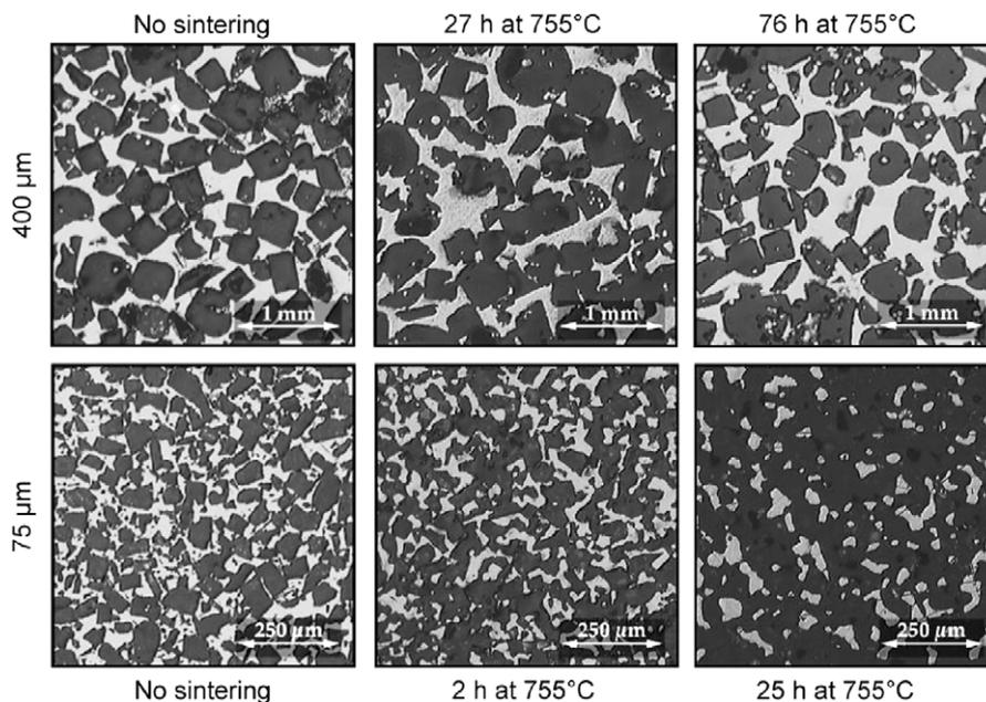
Fig. 1. Optical micrographs of polished sections through resin-infiltrated preforms of NaCl of 400  $\mu\text{m}$  and 75  $\mu\text{m}$  diameter, made by sintering at 755 °C for different periods of time. The dark phase is NaCl and the light phase is mounting resin.
