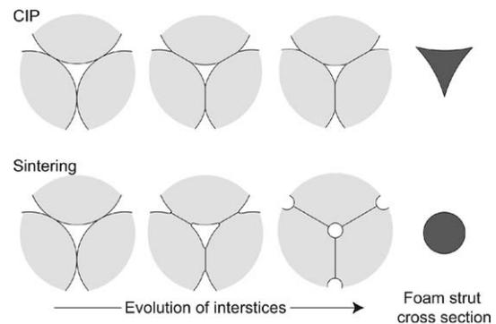
Fig. 5. A schematic diagram of three particles, showing a cross-section through the plane containing their centres, during sintering and CIP, illustrating the difference in the foam strut shapes produced.
