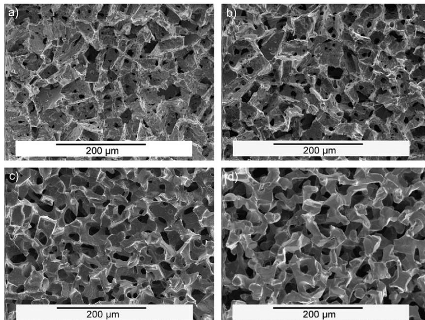
Fig. 3. Secondary electron SEM images of pure aluminium foams made by the replication method using preforms of 75  $\mu\text{m}$  NaCl particles: (a) unsintered ( $V_f = 0.4$ ), and sintered at 755  $^{\circ}\text{C}$  for (b) 2 h ( $V_f = 0.37$ ), (c) 9 h ( $V_f = 0.32$ ) and (d) 25 h ( $V_f = 0.25$ ).
