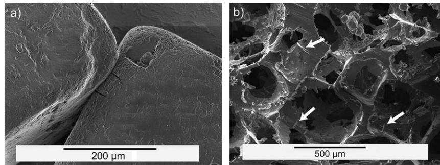
Fig. 2. Secondary electron SEM images of (a) the contact point between particles of 400  $\mu\text{m}$  NaCl after CIP at 28 MPa, and (b) the resulting foam after infiltration under 4 bar pressure ( $V_f = 0.2$ ), with replicated cracks indicated by the white arrows.
