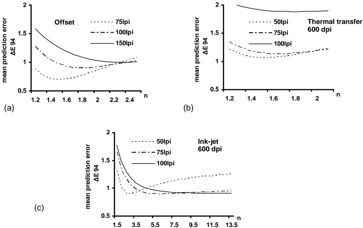
Fig. 4 Relationship between  $n$ -value and mean prediction error over 729 print samples for (a) offset prints on matte coated paper at 75, 100 and 150 lpi, (b) thermal transfer prints on calendered paper at 50, 75 and 100 lpi and (c) ink-jet prints on coated paper at 50, 75 and 100 lpi
