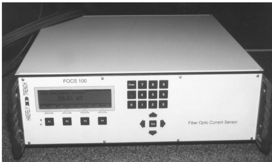
Figure 1: Sagnac fibre optics current sensor ready for field measurements. The sensing cable that must enclose the probed electrical conductor is partially shown on top-left of the figure.
