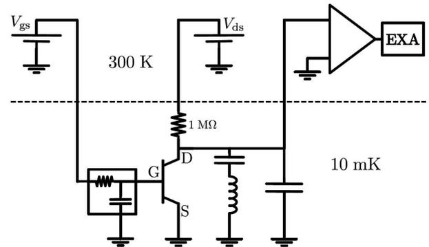
Fig. 1. Experimental setup for the measurement of low frequency noise (around  $388\text{kHz}$ ) for a channel of resistance  $10\text{k}\Omega$ . The capacitance symbol in parallel with the inductance represents the stray capacitance of the cable and the input capacitance of the amplifier. “EXA” refers to the Agilent spectrum analyzer.
