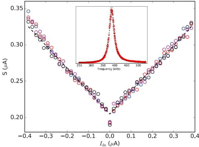
Fig. 2. Rescaled low frequency noise  $S/e$  of the conducting channel of the FET as a function of the dc bias current. The noise is measured at low frequency (388kHz) for a channel of resistance  $10\text{k}\Omega$ . The gate voltage is adjusted for each value of the drain-source voltage to keep the differential resistance of the channel constant. Inset: Example of voltage noise spectrum. The height corresponds to  $2.5 \times 10^{-17}\text{V}^2/\text{Hz}$ .
