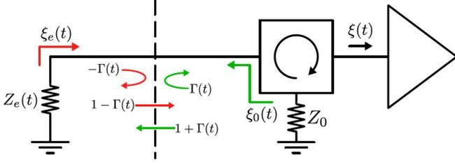
Fig. 5. Schematics of generation of vacuum squeezing by resistance modulation. Red arrows correspond to the noise generated by the modulated resistance  $Z_e$ . Green arrows correspond to the noise generated by the load of the circulator  $Z_0$ .
