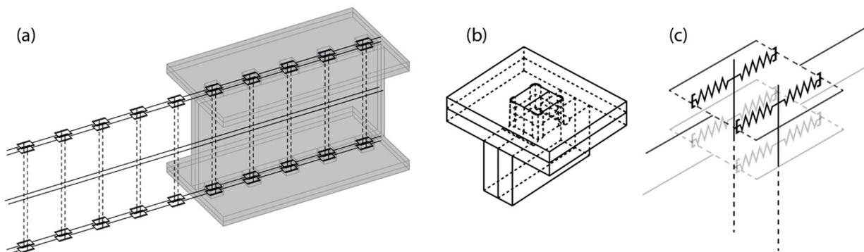
Figure 1: (a) representation of an I-Beam using wood-wood connections with the simplified calculation model (b) Axonometry of a TT joint (c) modelling of the TT joint with beam elements and springs.
